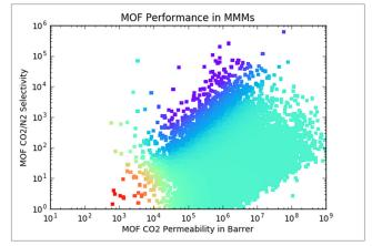
Calculated selectivity versus  $\mathrm{CO}_2$  permeability for a large database of MOF materials. Each point is colored based on the relative cost of carbon capture predicted for a hypothetical mixed matrix membrane made using that MOF. Cost is highest for red, moderately high for green, moderately low for blue and low for purple.
